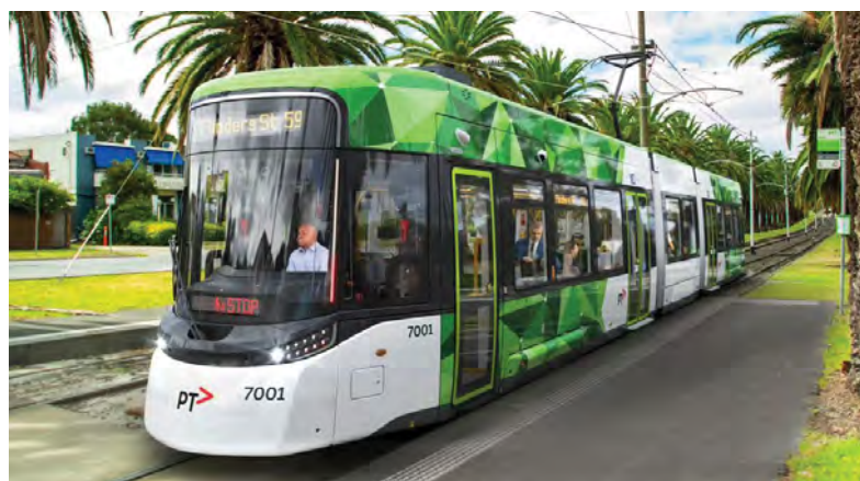
New low floor DDA compliant accessible G class tram, capacity 150 passengers
