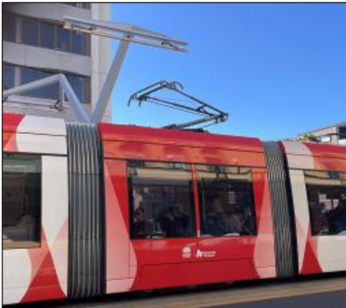
Newcastle - showing overhead Light Rail charging point.
