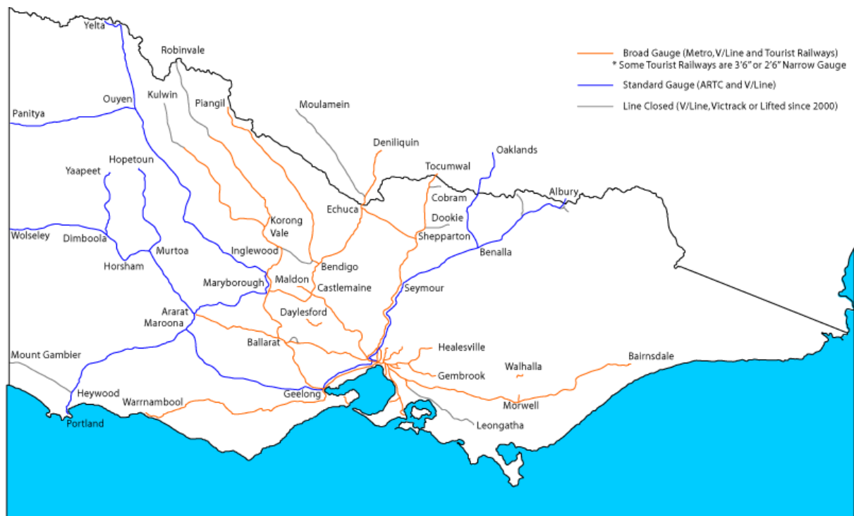
Figure 1: Victoria's regional rail system – it is not a network – showing the mix of standard gauge (1435 mm) and broad gauge (1600 mm) lines.
